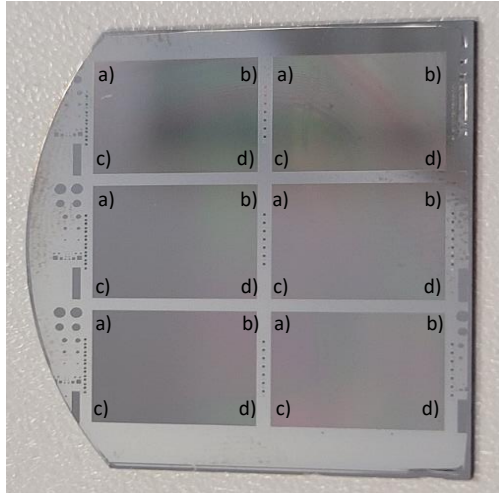
Figure 3 Etched 6 full arrays and discrete detectors on an appropriately cut piece of 2-inch GaAs wafer, using a photolithographic mask prepared for etching 2-inch GaAs structures, where the surroundings of each array are not the same.
